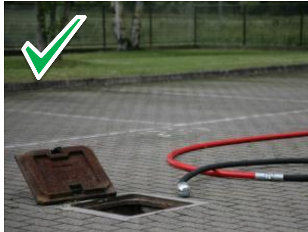
The ECOLEADER Sewer Leader Hose is a section of hose to be attached to the front of the main jetting hose.
