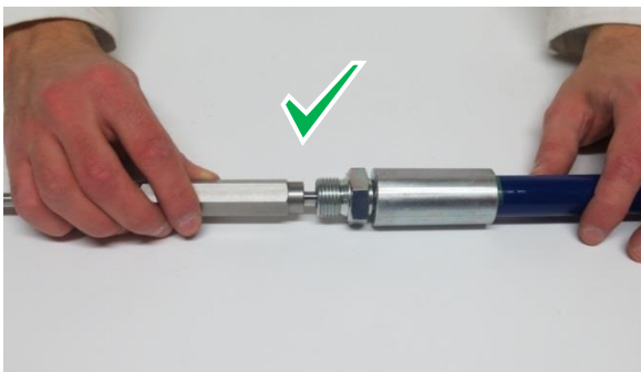
1. Go side must slide through the whole length of the insert
