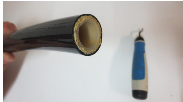
Use a proper tool to remove burrs and/or residual from the cut surface.
