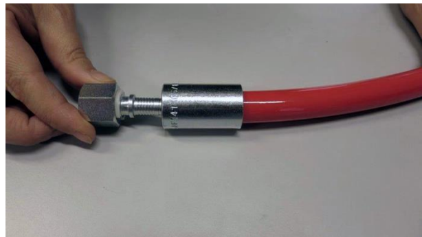
Marking the insertion depth of the ferrule and then put insert into the hose.
